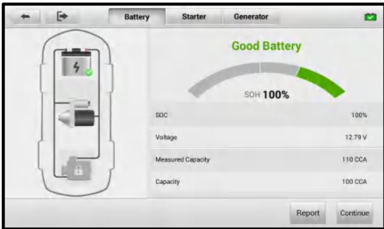
Figure 10-7 Battery Test Results Screen
