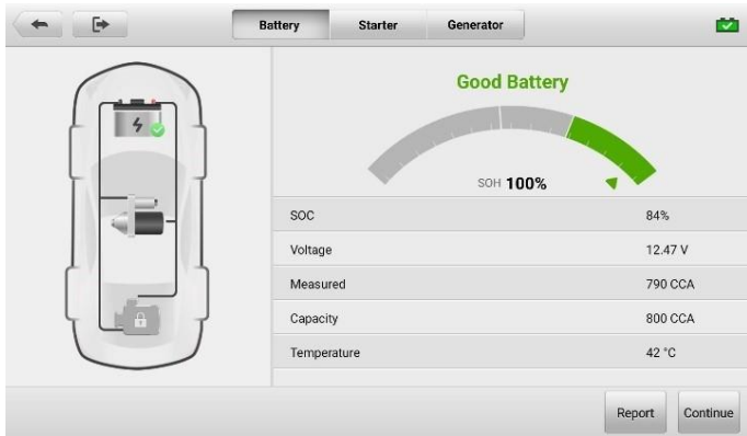
Figure 6-6 Battery Test Results Screen
